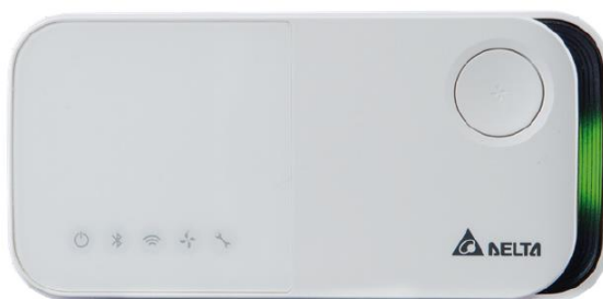
Figure 13: LOYUNO-L for indoor air quality monitoring.
