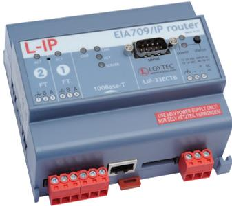
The L-IP Router connects twisted pair channels (TP/FT-10 or TP/XF-1250) with the Ethernet/IP channel (IP-852) in LonMark Systems. L-IP routes CEA-709 packets through an IP based network such as a LAN (Ethernet), an Intranet, or even the Internet. The L-IP connects to the IP network via a 100Base-T Ethernet port.
