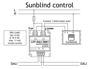
In Relay-Mode (operating mode 0x00) the module acts as DALI-2 certified relay module with 2 interlocked contacts: normally open and normally closed.
