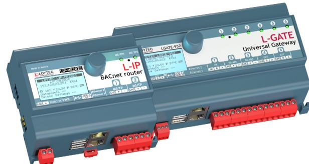
The L-IP Routers LIP-1ECTC, LIP-3ECTC, LIP-33ECTC, and LIP-3333ECTC connect twisted pair channels (TP/FT-10 or TP/XF-1250) with the Ethernet/IP channel (IP-852) in LonMark Systems. L-IP routes CEA-709 packets through an IP based network such as a LAN (Ethernet), an Intranet, or even the Internet.
