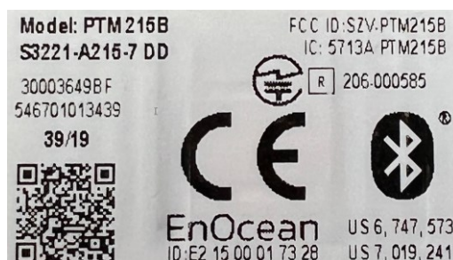
Figure 231: PTM215B label with ID (MAC-address) and QR-code.
