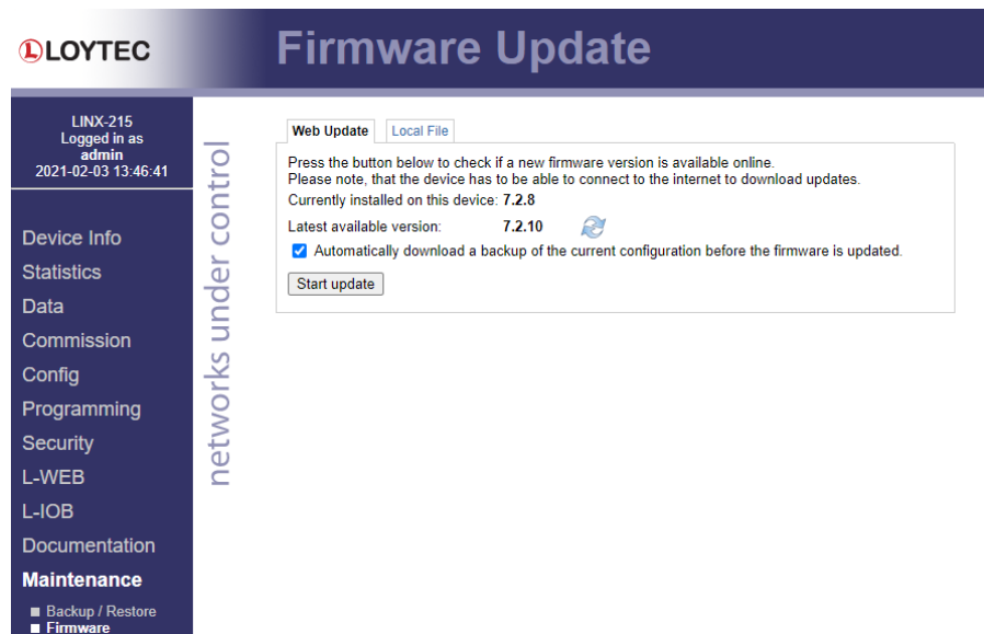
Figure 138: Firmware upgrade over the Web interface.
