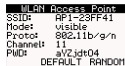
Figure 8: Access Point Setup on the LCD Display.
