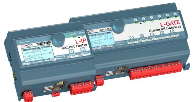
The L-IP Routers LIP-1ECTC, LIP-13-ECTC, LIP-3ECTC, LIP-33ECTC, and LIP-3333ECTC connect twisted pair channels (TP/FT-10 or TP/XF-1250) with the Ethernet/IP channel (IP-852) in LonMark Systems. L-IP routes CEA-709 packets through an IP based network such as a LAN (Ethernet), an Intranet, or even the Internet.
