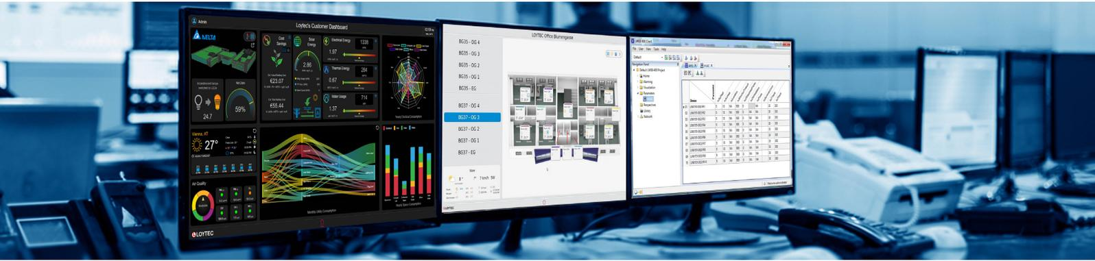
The L-WEB System is a powerful building management system platform for managing distributed building automation systems of any size. Maximum flexibility and scalability is achieved through the LWEB-900 client/server architecture in combination with the distributed LOYTEC L-INX Automation Servers and L-ROC Room Controllers.
