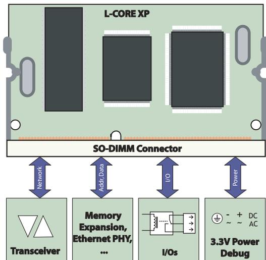
**Figure 2:** Block diagram of a typical network node using the L-CORE XP core module
