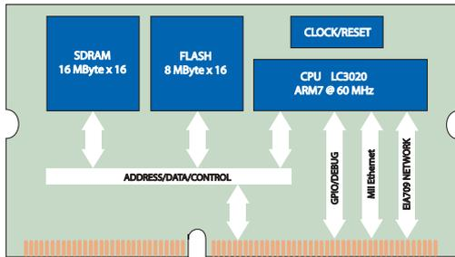
**Figure 1:** L-CORE-MOD block diagram.
