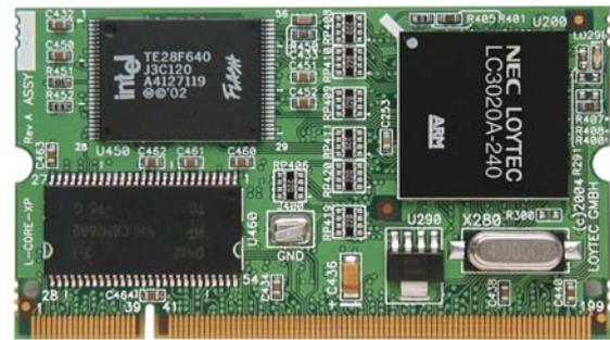
The L-Core XP philosophy is to provide a solution for building high-performance EIA-709 nodes at a very affordable cost. This can be achieved by either using the L-CORE XP module, a core module (SO-DIMM form factor!) that comes with a powerful ARM7 CPU LC3020, 8 Mbytes Flash memory, 16 Mbytes SDRAM, clock and reset circuitry, or by designing the L-Core components directly onto the target hardware.
