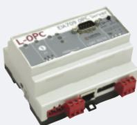
The LINX-110 Automation Server can manage any kind of application in a CEA-709 network. The device is programmed with the L-LOGICAD programming tool which is based on the IEC 61131-3 standard. The powerful logic can handle up to 1000 network variables (NVs) and up to 1000 address table entries to exchange data with a wide range of external controllers or I/O modules. LINX-110 features the complete set of automation functions.
