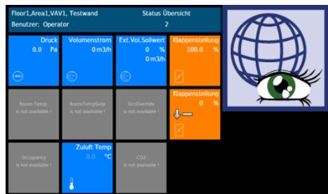
LWEB-803 is a graphical user interface to visualize dynamic pages showing plant details or a virtual room operator panel on a Microsoft Windows PC.
