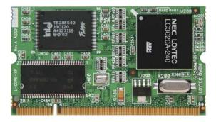
The L-Core XP philosophy is to provide a solution for building high-performance EIA-709 nodes at a very affordable cost. This can be achieved by either using the L-CORE XP module, a core module (SODIMM form factor!) that comes with a powerful ARM7 CPU LC3020, 8 Mbytes Flash memory, 16 Mbytes SDRAM, clock and reset circuitry, or by designing the L-Core components directly onto the target hardware.
