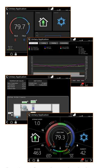
Figure 6: Automatically generated monitor and control graphics
