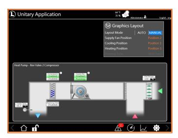
Figure 6a: Custom mode - reposition components such as fan and coil positions for custom renderings
