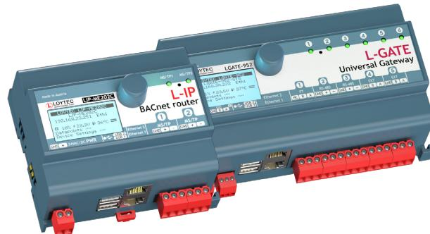
The L-IP Routers LIP-1ECTC, LIP-3ECTC, LIP-33ECTC, and LIP-3333ECTC connect twisted pair channels (TP/FT-10 or TP/XF-1250) with the Ethernet/IP channel (IP-852) in LonMark Systems. L-IP routes CEA-709 packets through an IP based network such as a LAN (Ethernet), an Intranet, or even the Internet.
