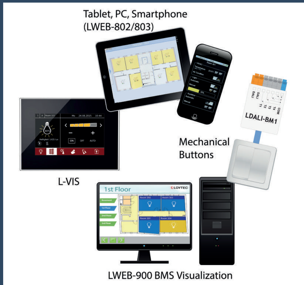
The L-DALI System offers a wide selection of operator interfaces.
