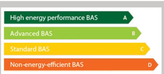
**Fig. 1: BAS efficiency categories for buildings according DIN EN 15322. Today's standard of newly constructed buildings only reaches category C.**
